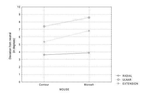
Figure 8: Average wrist deviation for the Contour and Microsoft ergonomic mice Although deviation for each posture is below the 30% excessive limit, the maximum deviation was above 30%.
