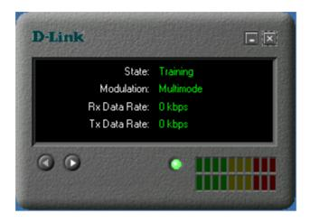
The bright green light under the screen indicates a valid link. The screen indicates the current state of you modem, the modulation and the Rx and the Tx data rates. On startup, the modem will automatically "train", or load the settings in your modem. Shortly after the training process, the screen below will appear, now showing your state as (receiving) Data.
