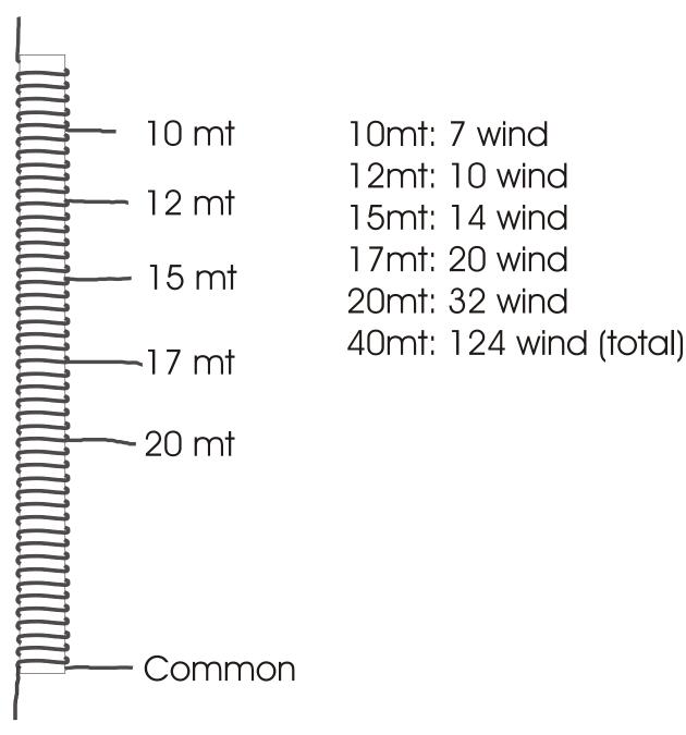
Whole coil is 1mm insulated wire closewound on 25mm diameter PVC support
