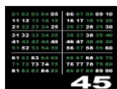
The programming tech is brought to the extremes, since displaying 90 small numbers on a screen (using a 512 lines assembler program) is a tough task even for a fast microcontroller as the Atmel's AVR AT90S1200. The (admittedly dirty) code and the schematic are derived from the **video-cronograph** project, cutting off the serial port output and the photocells input, so don't be surprised if you find some strange variable names.
